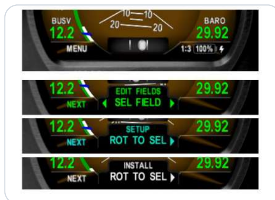
Figure 2 · Field sequence in the installation menu
