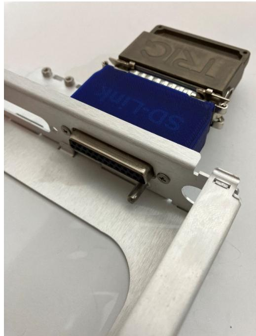
5. Connect the SD-TY96-DS adapter to the TRIG connector by joining the adapter's clips with the installed retaining clips of the TRIG connector.
