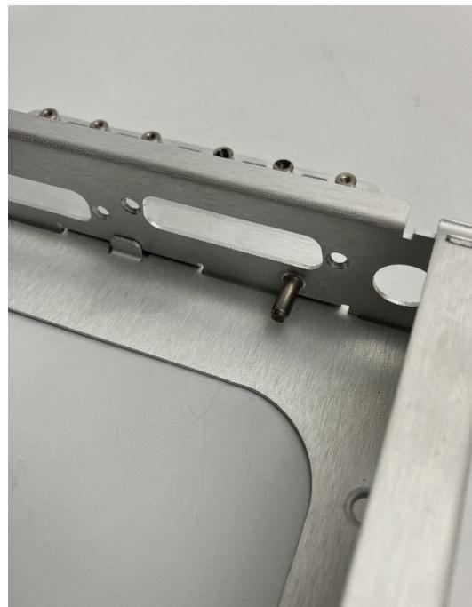
1. Remove the two Phillips head screws to detach the TRIG connector from the radio's tray.
