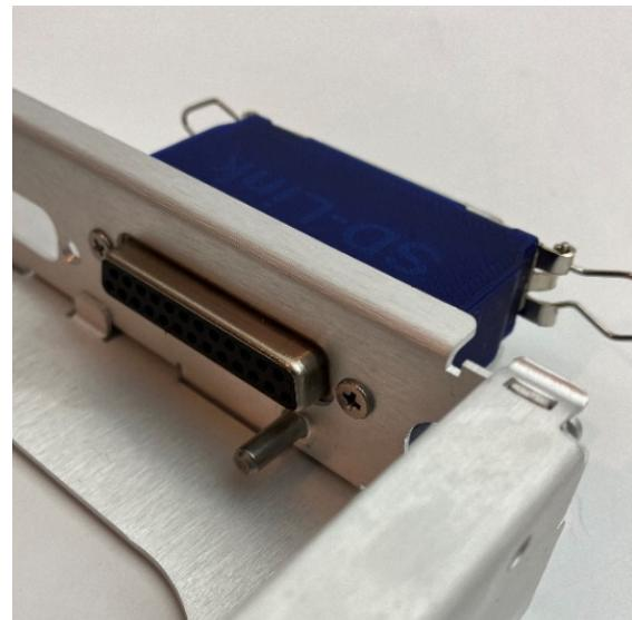
3. Install the SD-TY96-DS adapter into the tray using the included countersunk Phillips head screws (3 x 8 mm, for thermoplastics). Tighten the screws hand-tight and be careful not to overtighten the threads!
