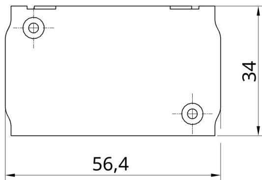
Bluetooth Low Energy Adapter (BLE) for a TRIG TY96/97 VHF transceiver (aviation radio). The adapter was developed as an interface between a TRIG TY96/97 and the navigation software SkyDemon (SD). It implements the data transfer between the navigation software (SD) and the radio hardware (BLE  $\leftrightarrow$  RS-232). The adapter is simply screwed between the radio's mounting rack and the existing connector.
