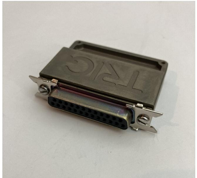
4. Mount the included retaining clips to the TRIG connector by tightening the UNC-4-40 screws with a slotted screwdriver.
