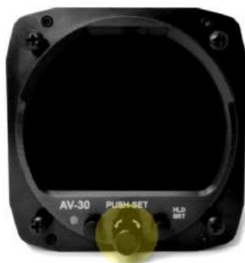
Figure 28 - Installation Menu Access
