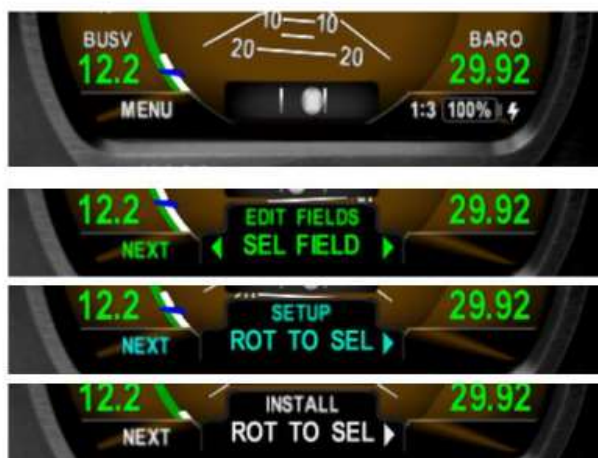
Figure 29 - Installation Menu Access
